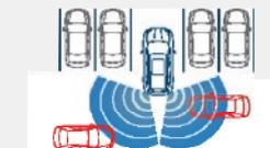
**Rear Cross-Traffic Alert**<sup>16</sup> alerts you with an audible warning and a flashing indicator on your side mirror and Rear-View Camera display if it senses traffic approaching from the side as you are backing up.
