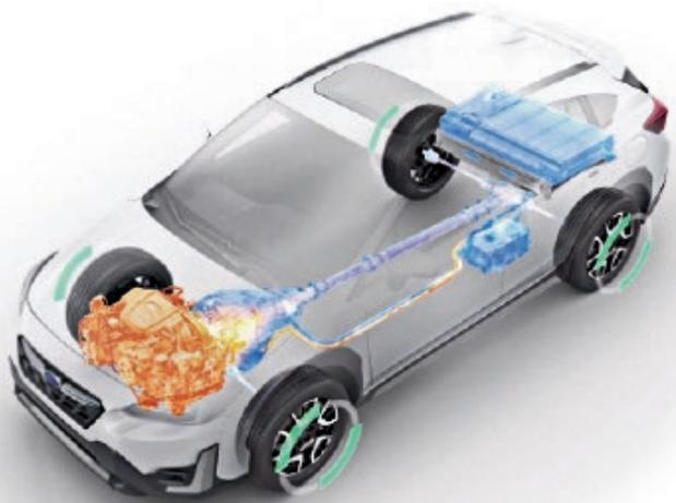
In **everyday driving**, the system will run on a combination of electric and gas power. It can also recover energy via regenerative braking.
